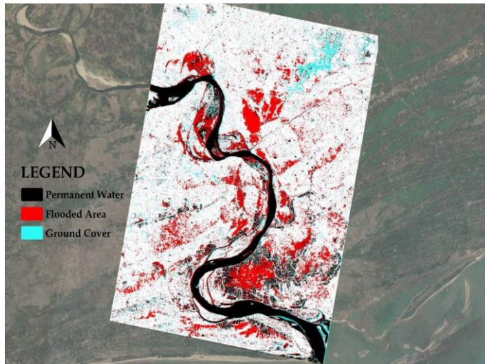
Figure 4 FLOOD HAZARD MAP FOR THE STUDY AREA (SUBARNAREKHA RIVER BASIN, ODISHA, INDIA). DERIVED FLOOD MAP FOR 29 MAY, 2021 FROM SENTINEL-1 SATELLITE IMAGE.
